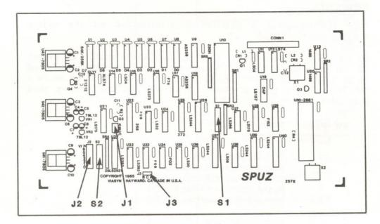
Figure 2. SPUZ (jumper and switch location)
