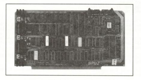
HIGH PERFORMANCE Z80 64 or 256K RAM DUAL ASYNCHRONOUS COMMUNICATION CHANNELS SPUZ TECHNICAL MANUAL Copyright 1985 Viasyn Corporation Hayward, CA 94545
