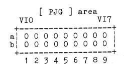
As an example, to connect Slave Interrupt Request to VI1, connect a jumper from a2-to-b2.
