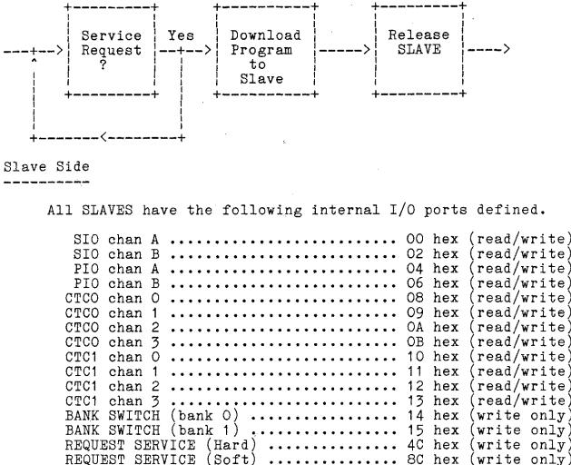
NOTE: The Slave internal I/O ports can not be read or written by the Master CPU.
