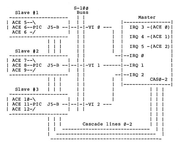
In the configuration above, the master Mult I/O board should have it's interrupt request pad (J5-B) connected to the PINT/ line of the buss, while slaves should have this pad jumpered to the appropriate VI lines. Slaves should also have all three board traces beneath the pads marked C, D and E in J5 cut open.
