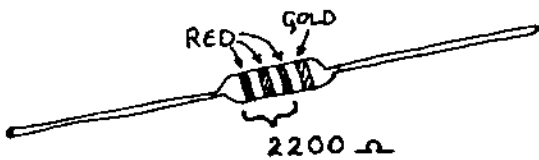
Carbon Film Resistor 5% (gold), 10% (silver)
