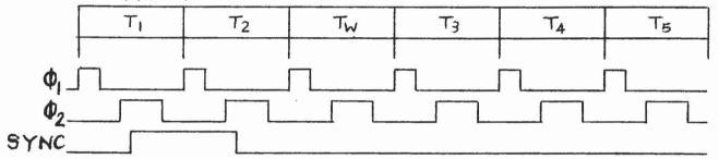
Dual-D flip flop U67 is used to set the number of wait cycles the CPU goes through when reading or writing data on this board. It signals that it is ready to read or write by actuating the Ready line (PREADY).
