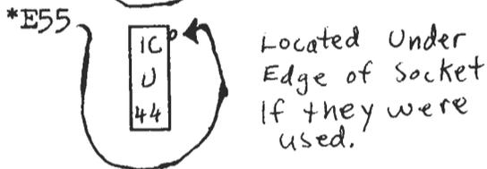
\* On first run boards (model 1011) These pads are already connected by a trace.
