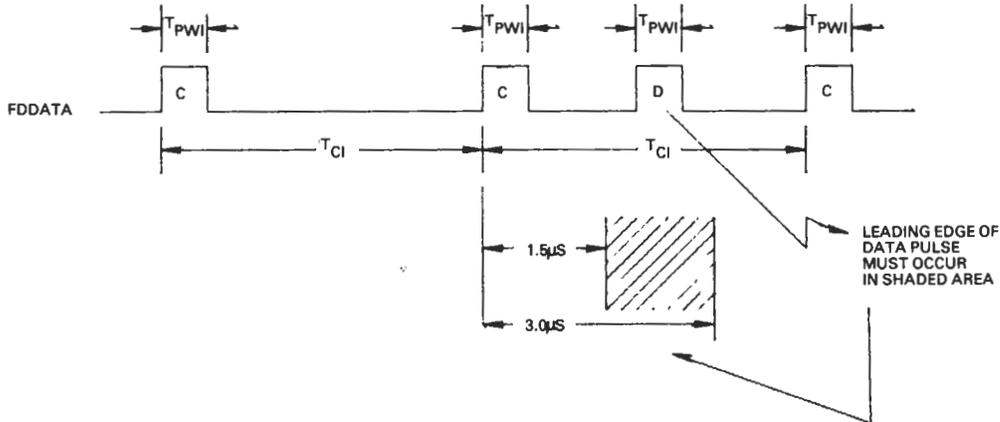
NOTE: INTERNAL DATA SEPARATION MAY WORK FOR SOME APPLICATIONS. HOWEVER, FOR APPLICATIONS REQUIRING HIGH DATE RECOVERY RELIABILITY, WDC RECOMMENDS EXTERNAL DATA SEPARATION BE USED.
