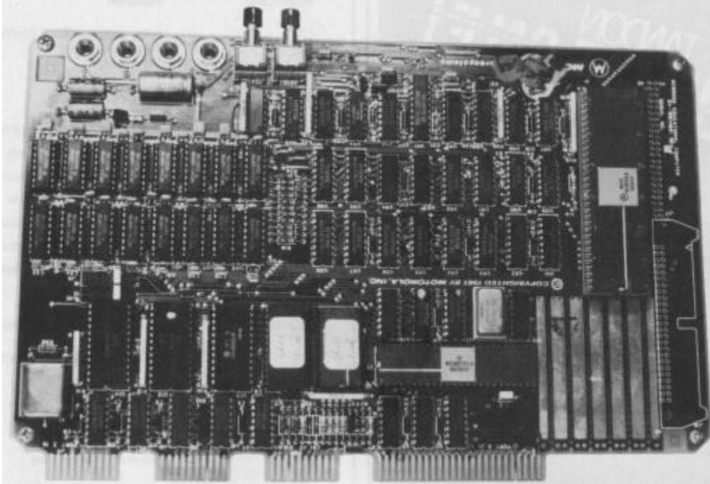
**Photo 1:** The very large integrated circuit (IC) in the upper right is the 68000. The other large IC near the wire-wrap area is the 48-pin MC68230 parallel interface/timer. The two serial interface ICs are at lower left. The edge connectors on the bottom are, from left to right, serial port 2 (host), serial port 1 (terminal), port 4 (cassette recorder), and port 3 (Centronics-type parallel printer).
