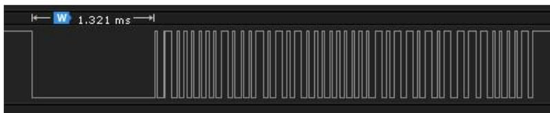
Notice that the pulling low of the line actually lasts 1,3ms which is a bit on the long side but does no harm.
