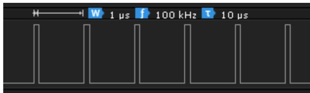
As an alternative to setting the pulse width we can specify percentage of the period that the pulse is high. This is called the duty cycle. For example, a duty cycle of 50% means the pulse is high for half the period and we have a perfect square wave. A duty cycle of 0% is always low and 100% is always high.
