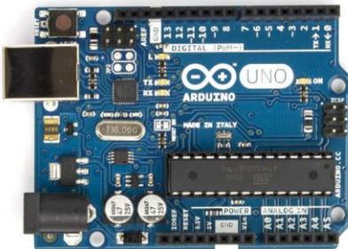
The key feature of the Arduino is that it is simple but very expandable. It doesn't have a full operating system and it doesn't have a video/keyboard interface. It supports a range of digital and analog I/O as standard.
