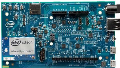
The Arduino breakout board is easy to use. Especially so if you already have Arduino experience. The reason is that one of the possible programming environments for the Edison is the Arduino IDE which allows you to write programs as if you were working with a real Arduino.
