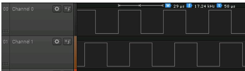
You can see that the pulse trains are not 180 degrees out of phase. The top train switches on and the bottom train takes about half a pulse before it switches off - the intent is for both actions to occur at the same time. The point is that it does take quite a long time to access and change the state of an output line.
