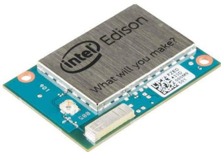
The Edison is a full computer, but without a video or keyboard interface. This means you have to work with it via a remote console - either connect via a serial/usb or network connection. Connections to the outside world can be via the built in WiFi, BlueTooth, serial port or USB. Even though it runs Linux it doesn't have a desktop environment only a command line.
