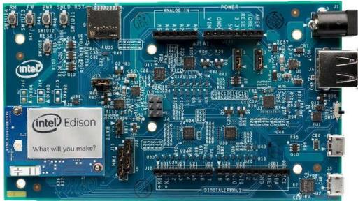
However, the [Edison](#) plus the Arduino breakout board isn't exactly an Arduino - it is more than an Arduino because it is a full Linux machine as well. So there are many new things to learn.
