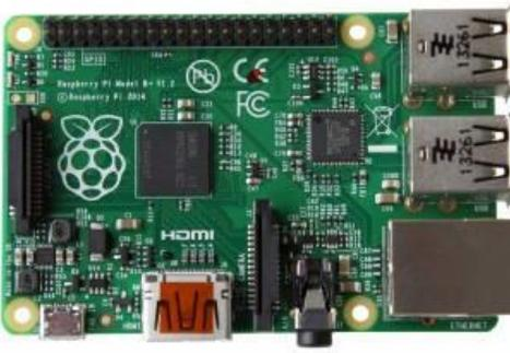
The Pi is a full computer that just happens to have a GPIO interface that you can use to control the real world. It has a video display and keyboard interface and you can use it standalone just like any machine - though it is common to use another PC to configure and program it via a remote console or desktop.
