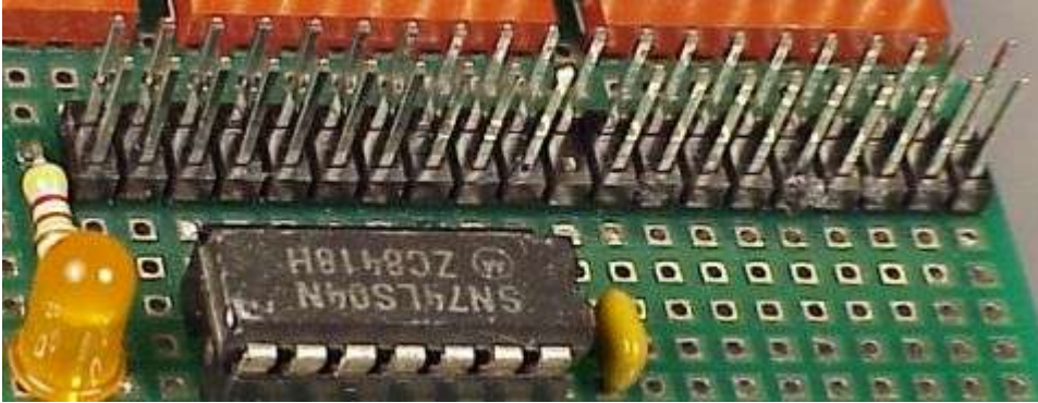
Figure 2: IDE Interface Circuit. Very few parts are needed. Pin 1 is located at the upper right. Pin 20 is removed. Had a connector with a polarizing notch been used, the notch would appear at the top of this picture, opposite the even numbered side, with pin 20 removed.
