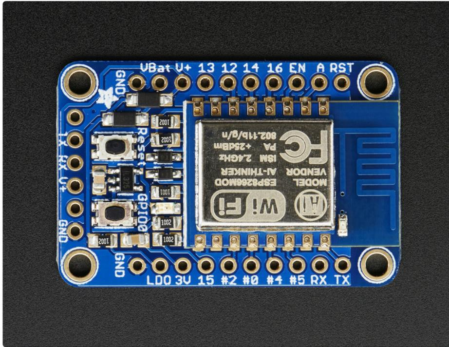
The HUZAZH ESP8266 breakout is what we designed to make working with this chip super easy and a lot of fun. We took a certified module with an onboard antenna, and plenty of pins, and soldered it onto our designed breakout PCBs. We added in:
