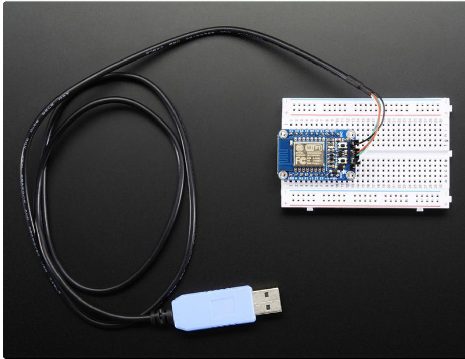
Each module comes pre-loaded with NodeMCU's Lua interpreter (NodeMCU 0.9.5 build 20150318 / Lua 5.1.4 to be specific) (<https://adafruit.it/inA>), you can run commands, and 'save' Lua programs directly to the module's Flash using a USB-Serial converter cable.
