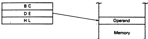
Figure 90. Register Indirect Addressing
