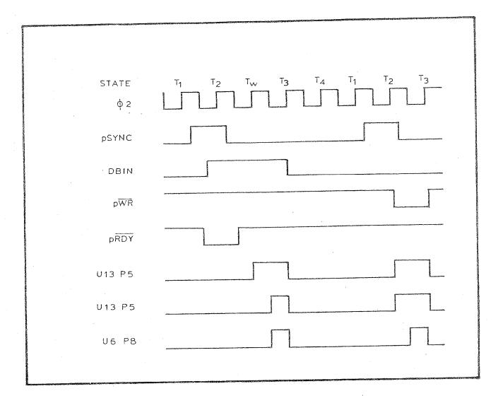
As an example, consider the sequence of events during an address breakpoint on input port number FF while running the FF PORT TEST PROGRAM.
