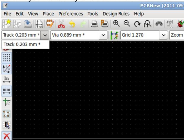
16. If you would like to add more track widths go to: **Design Rules** → **Design Rules** → **Global Design Rules** tab and at the bottom right of this window add any other width you would like to have available. You can then choose the widths of the track from the drop-down menu while you lay out your board. See the example below.
