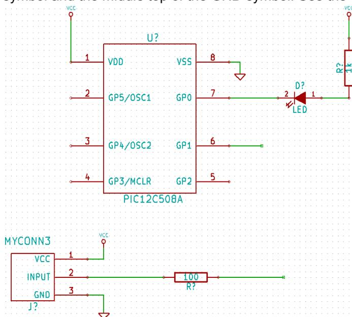
32. We will now consider an alternative way of making a connection using labels. Pick a net labelling tool by clicking on the 'Place net name' icon
